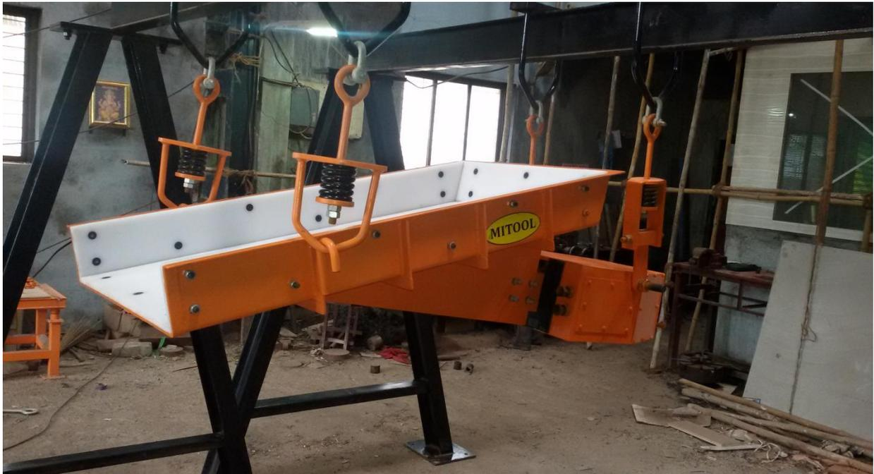
Mitool Make Vibrating feeders are most efficient & economical to convey the bulk materials & in the simplest easiest means of controlling the flow rate.
